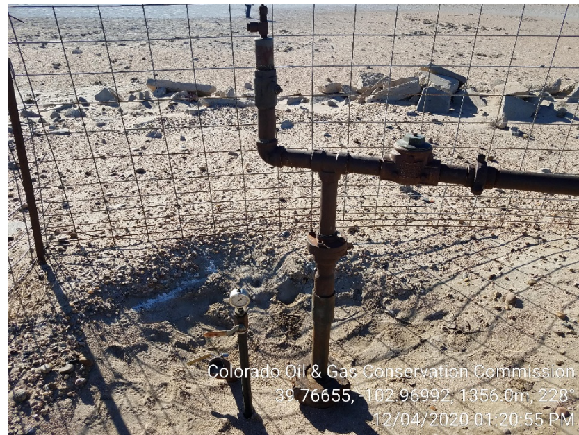
2. Wellhead/Braidenhead riser
