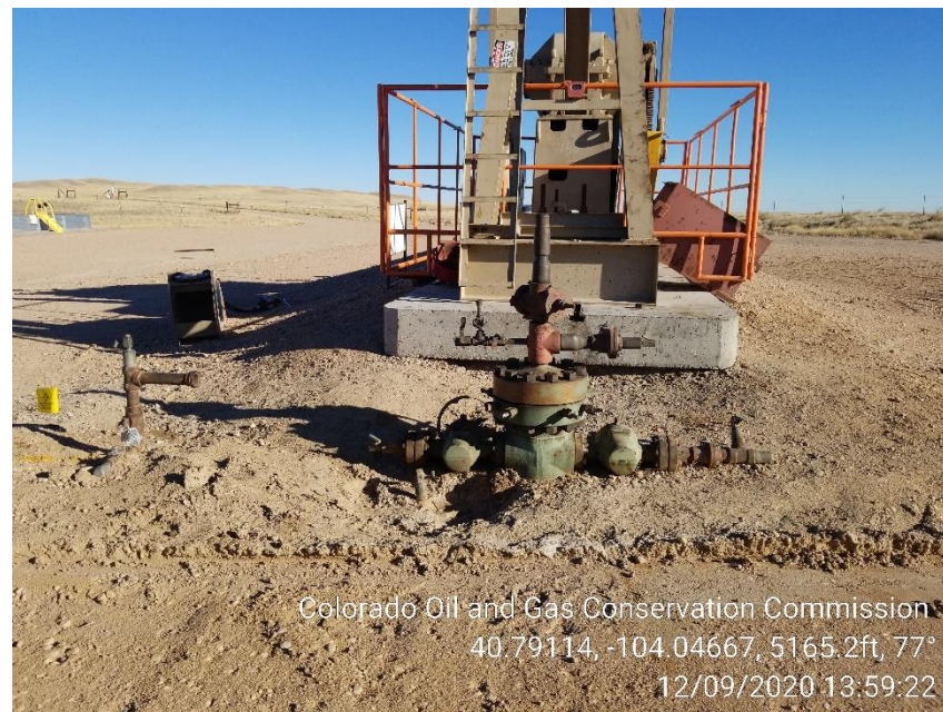
Photo 2 – Wellhead, Stained Soil cleaned up
