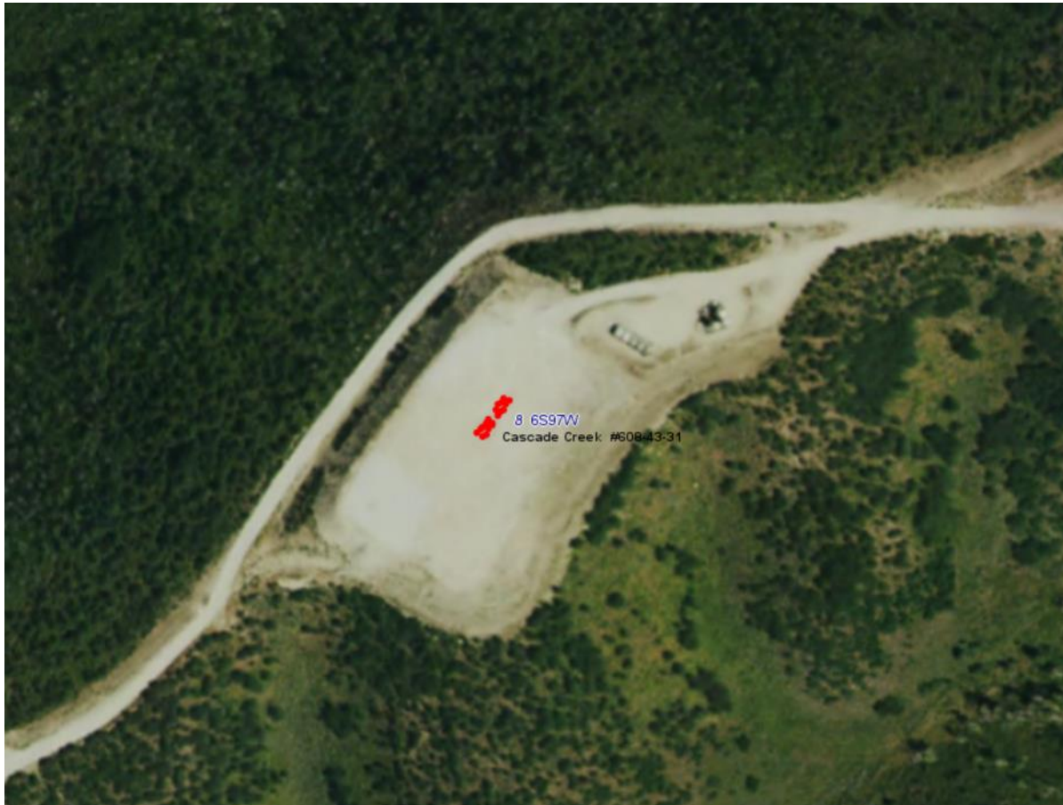
Photo 1: 2019 COGIS Aerial imagery. Photo shows areas not reasonably needed for production on the Location have not been reclaimed.
