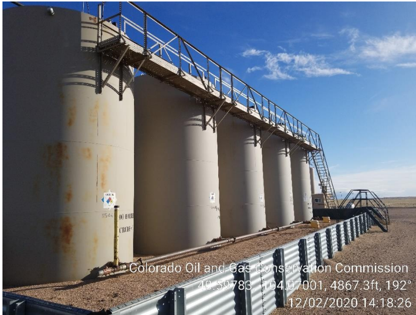
Photo 1 – Tank Battery
