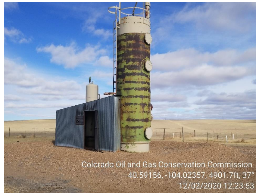
Photo 2 – Unused Heater Treater and Vertical Separator
