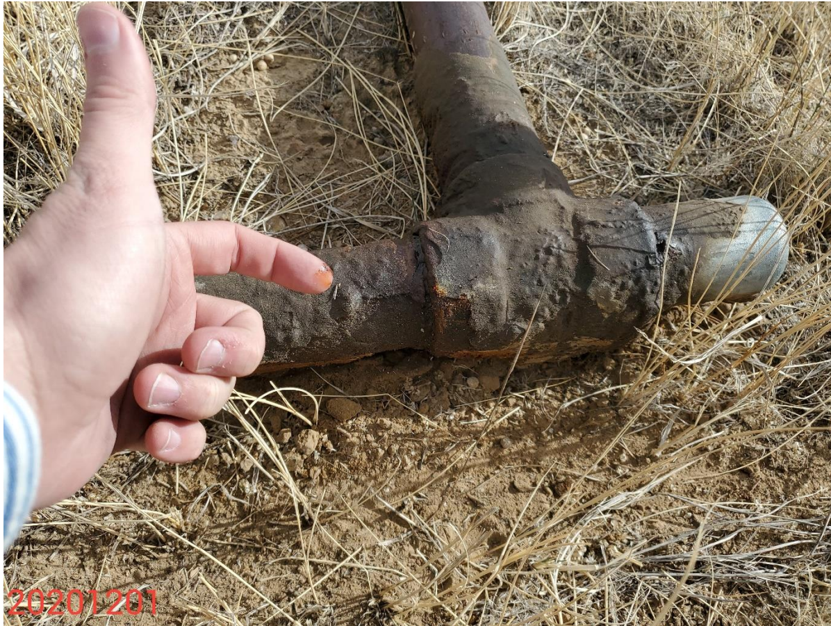
Photo 5: Continued from photo 4. Photo shows leaking from the flowline remains evident. Maintenance to prevent failures or leakage has not been conducted
