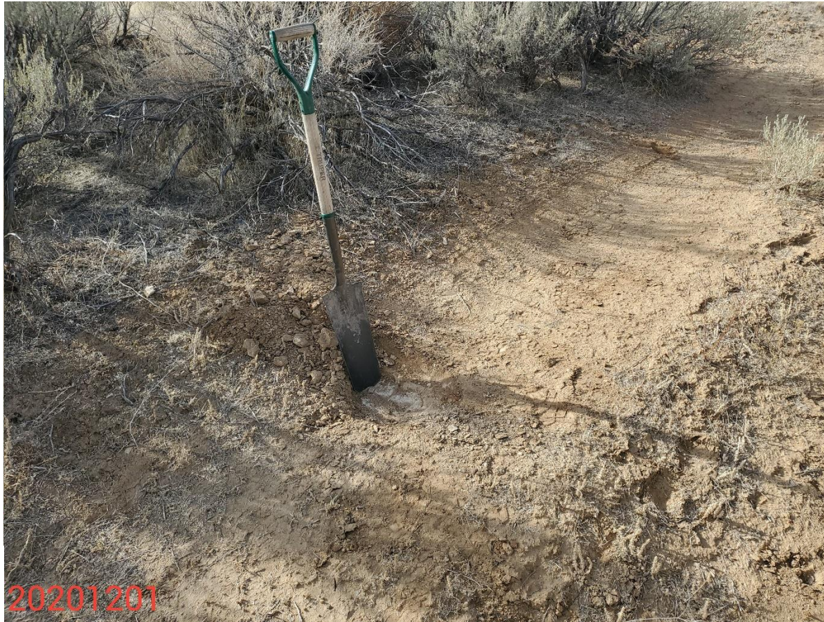
Photo 9: Photo taken from the access road. Photo shows a test pit on the access road to determine compliance with compaction alleviation requirements. Soils at the surface was fairly loose and easy to penetrate. Compaction zones were encountered ~2-3 inches subsurface. Reclamation of the access road has not been conducted in accordance with 1004 requirements.
