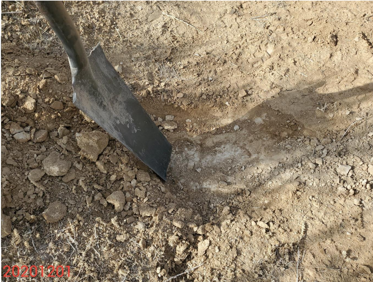
Photo 10: Continued from photo 9. Photo shows compacted soils exist ~2-3 inches subsurface.
