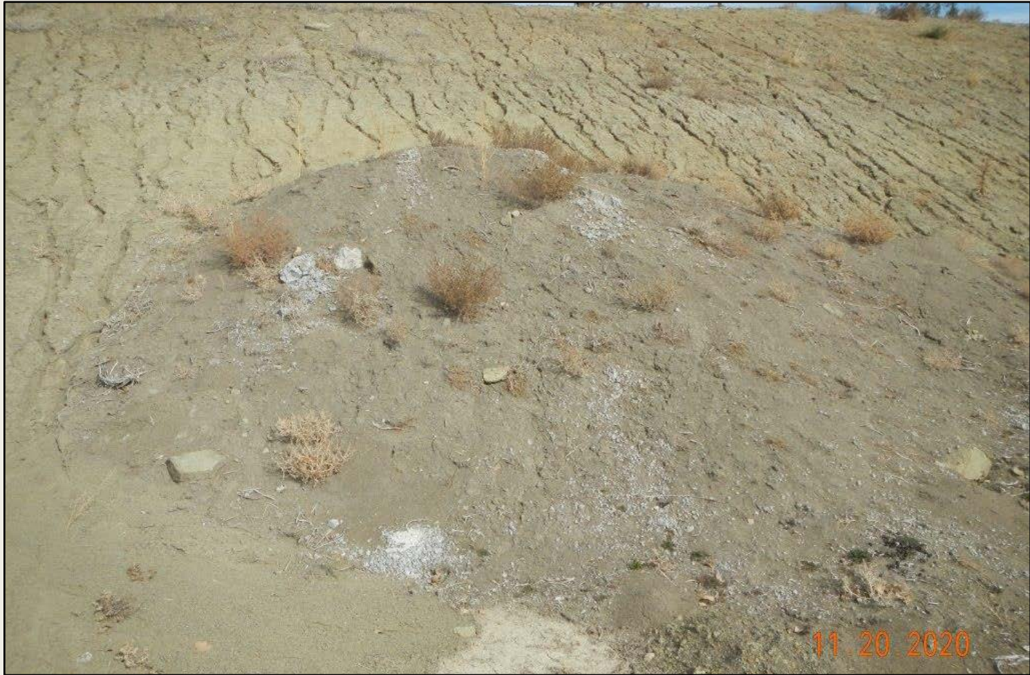
Photo 4. View of unknown soil material that appears to be cuttings, placed at the base of the cut-slope.
