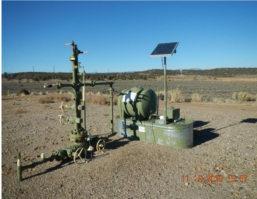
Ignacio 33-7 #19A well head and chemical injection system.
