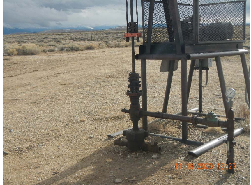
Photo 2. No bradenhead access apparent.
