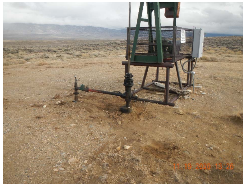
Photo 2. No bradenhead access apparent.
