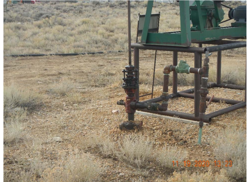
Photo 2. No bradenhead access apparent.
