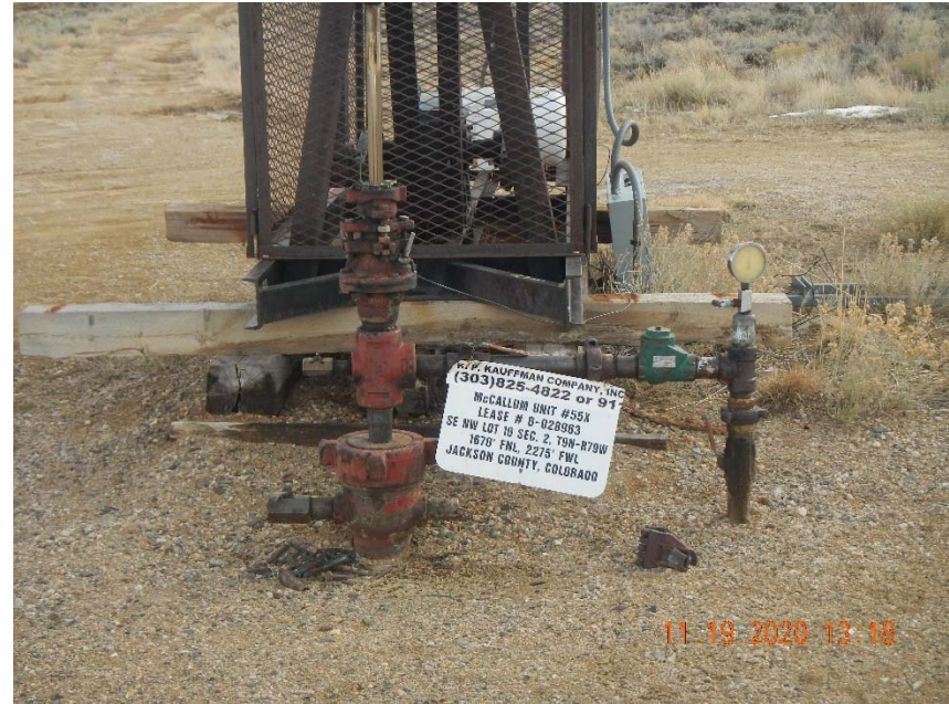
Photo 2. No bradenhead access apparent.
