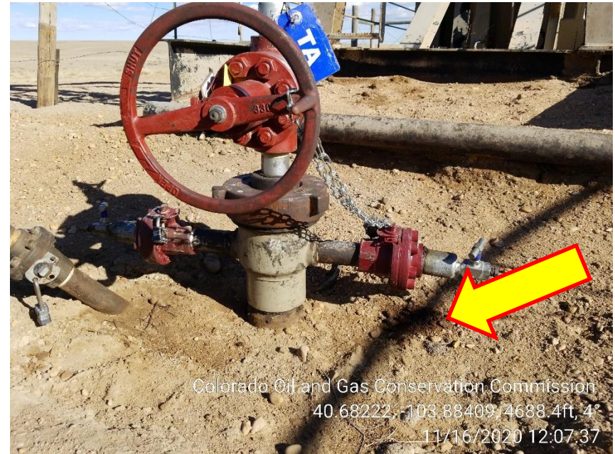
Photo 2 – Wellhead, Stained Soil
