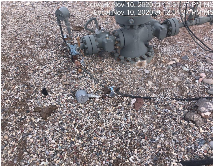
Photo #2231 Braden head valves are not accessible on well 17-14A.
