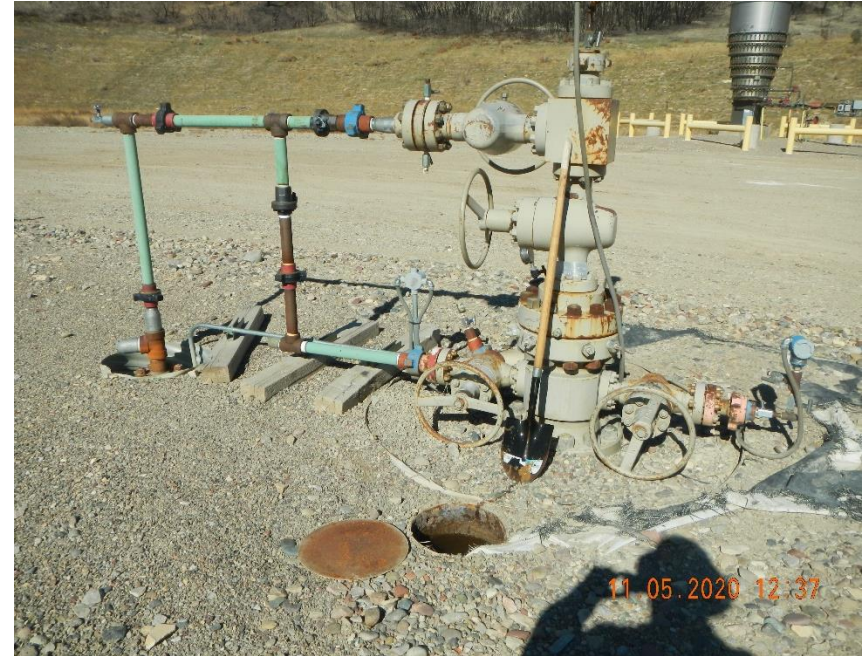
Shovel used to check for backfill.
