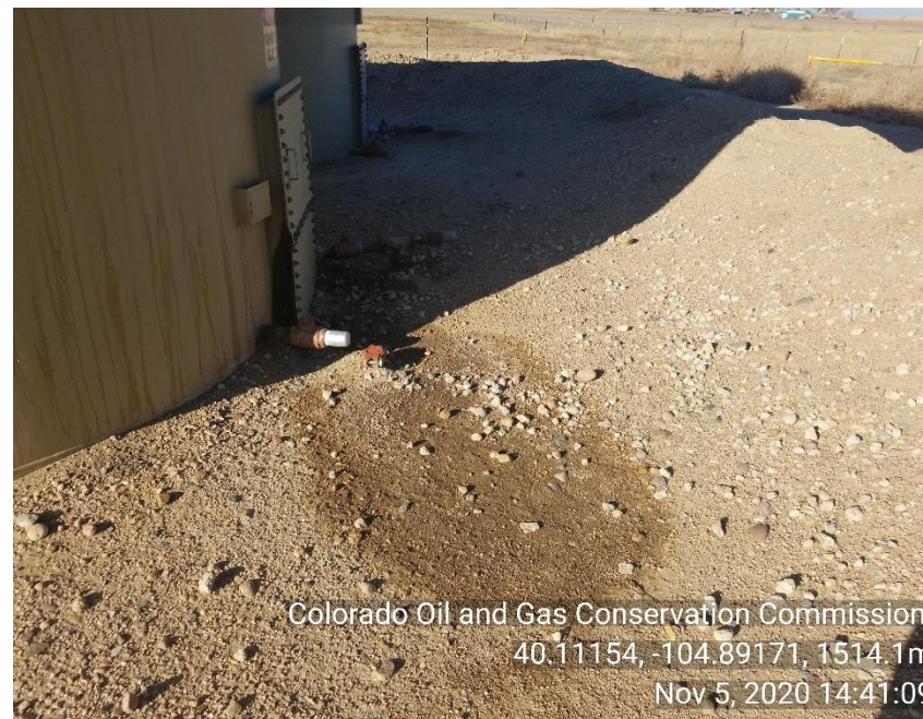
Photo 11 Stained soil from leaking 2" crude oil line.
