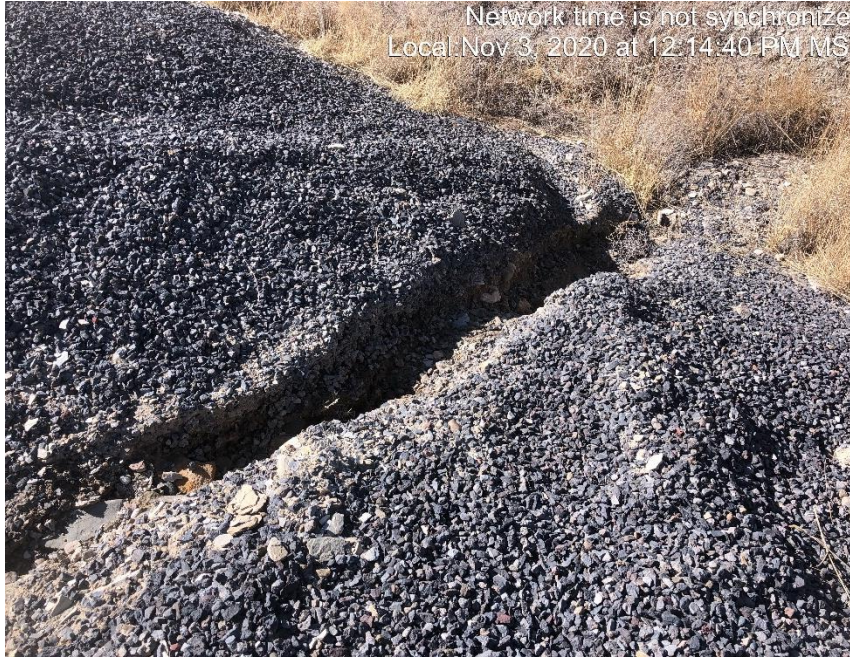
Photo #2174 Rill erosion occurring on west end of location
