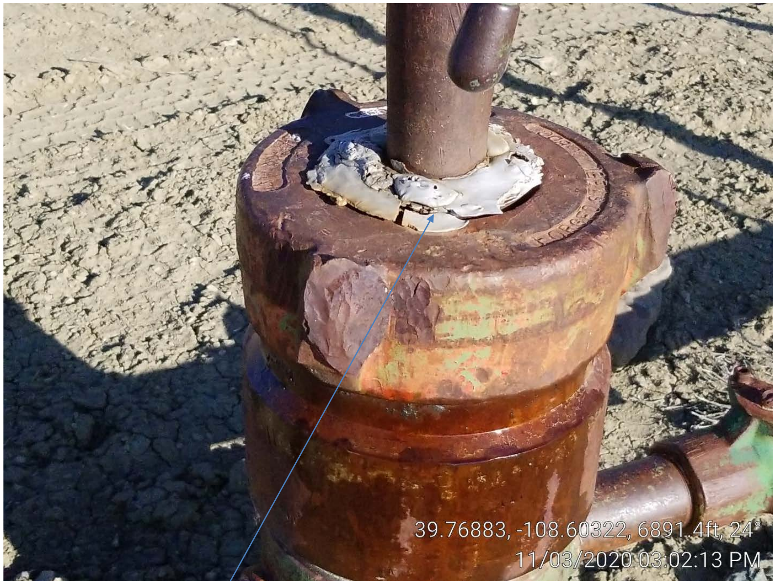
Photo 4. Gas leak at well.
