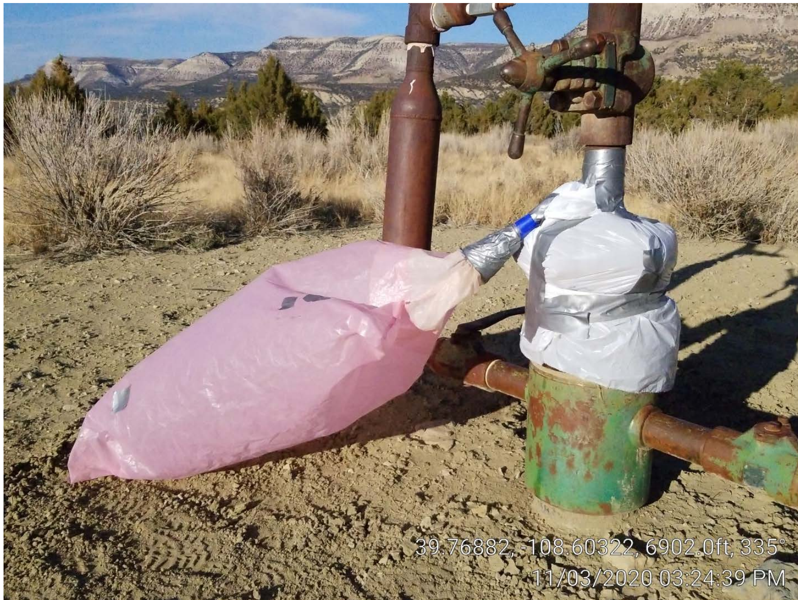
Photo 5. Bag attached to well gas leak.
