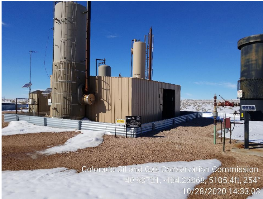
Photo 1 – Heater Treaters
