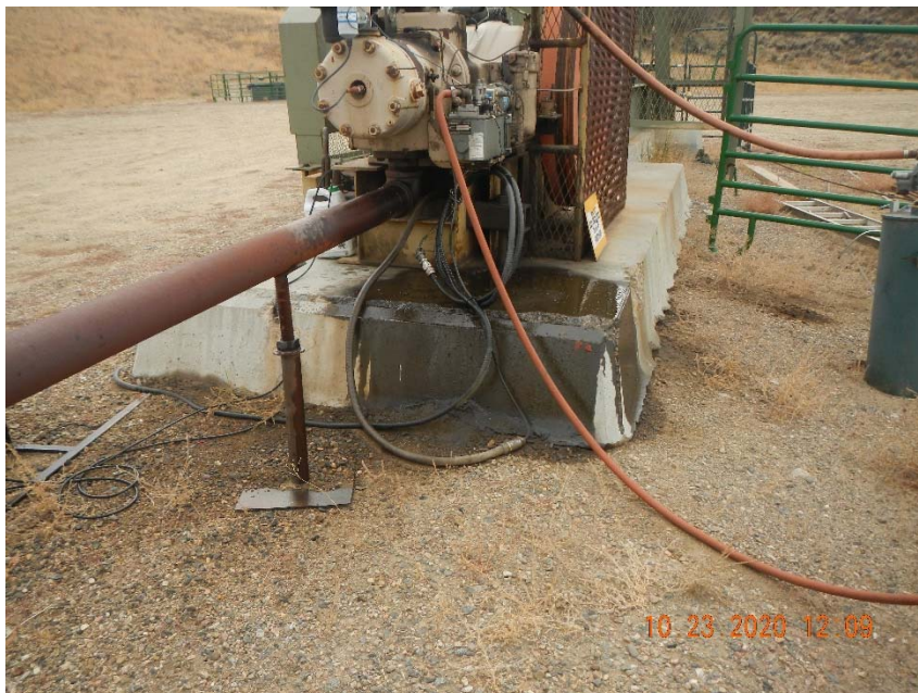
Photo 2. Stained soil at pump jack.
