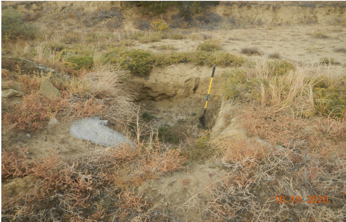
Photo 4. There is an open hole which is about 4.5 ft. deep shown by shovel placed in the hole. There is cement debris next to the hole which appears to be from plugging the well.
