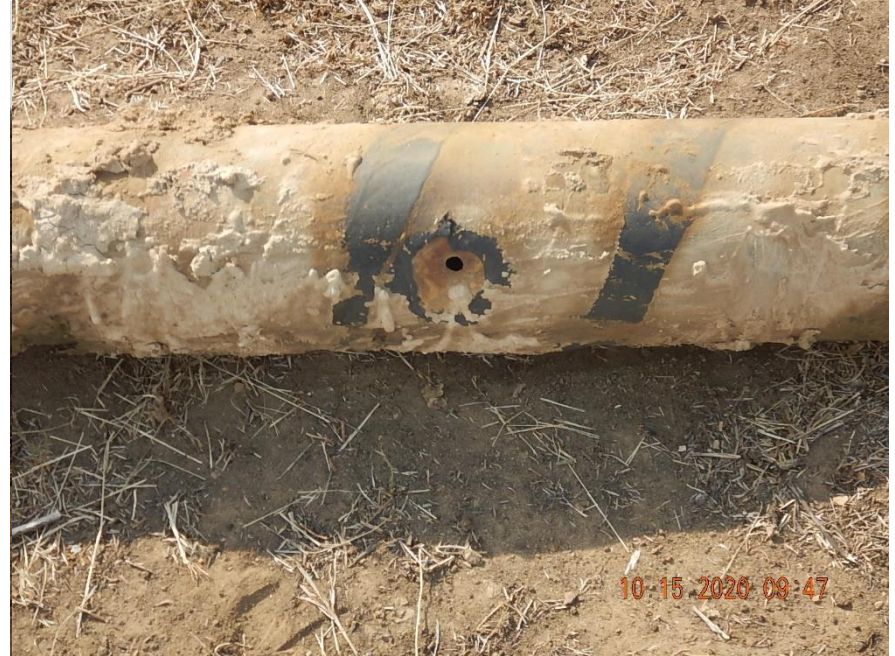
External corrosion hole identified in the side wall of the carbon steel flowline segment removed from the excavation.
