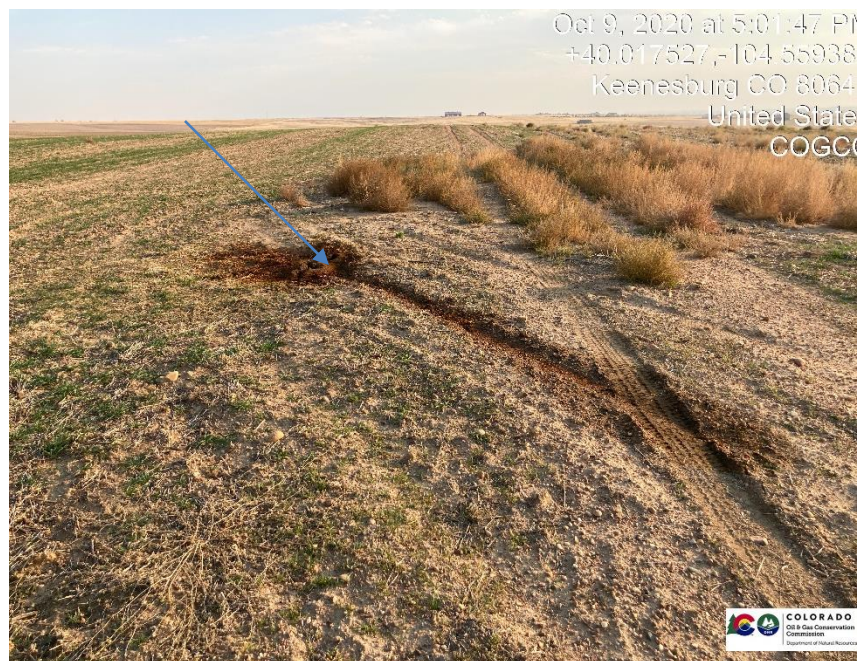
Pic 1 Stained soil, and gas venting from ground looking south.
