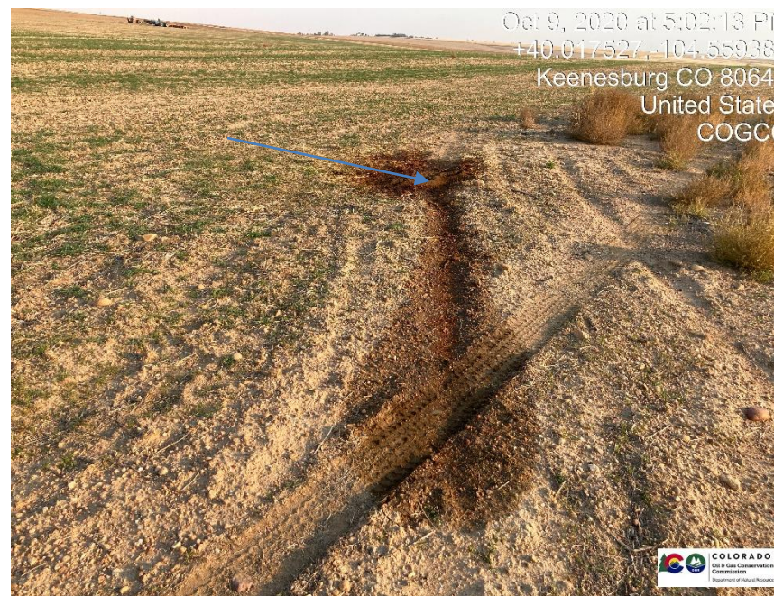
Pic 2 Stained soil, and gas venting from ground looking south.
