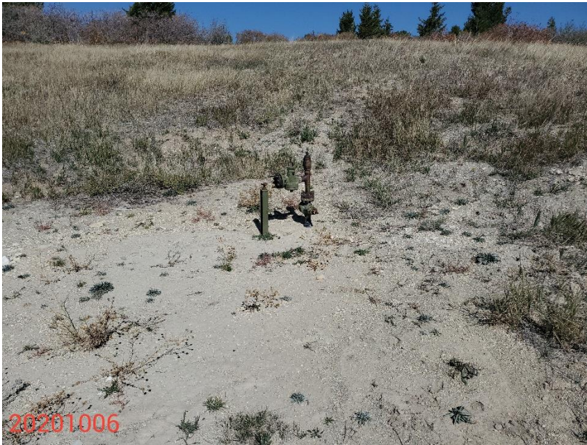
Photo 5: Photo taken from the northeast corner of the Location. Photo shows Pipe riser surface equipment remaining on the Locaiton.
