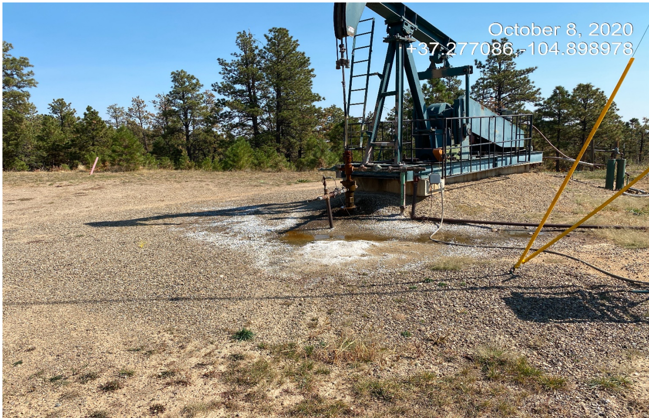
Photo 2. There is water leaking at the wellhead.
