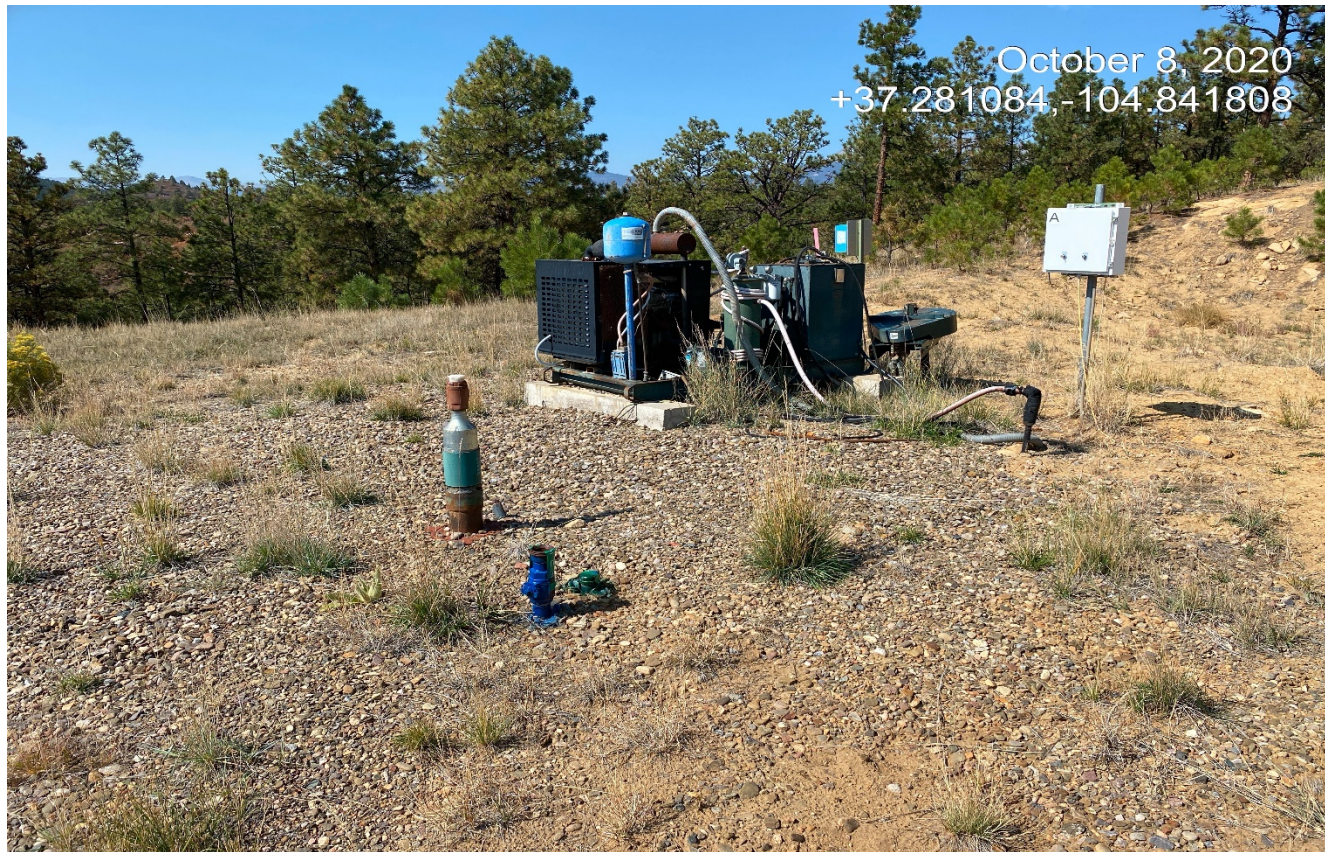
Photo 6. Well is temporarily abandoned. Unused equipment and pipe risers need to be removed.
