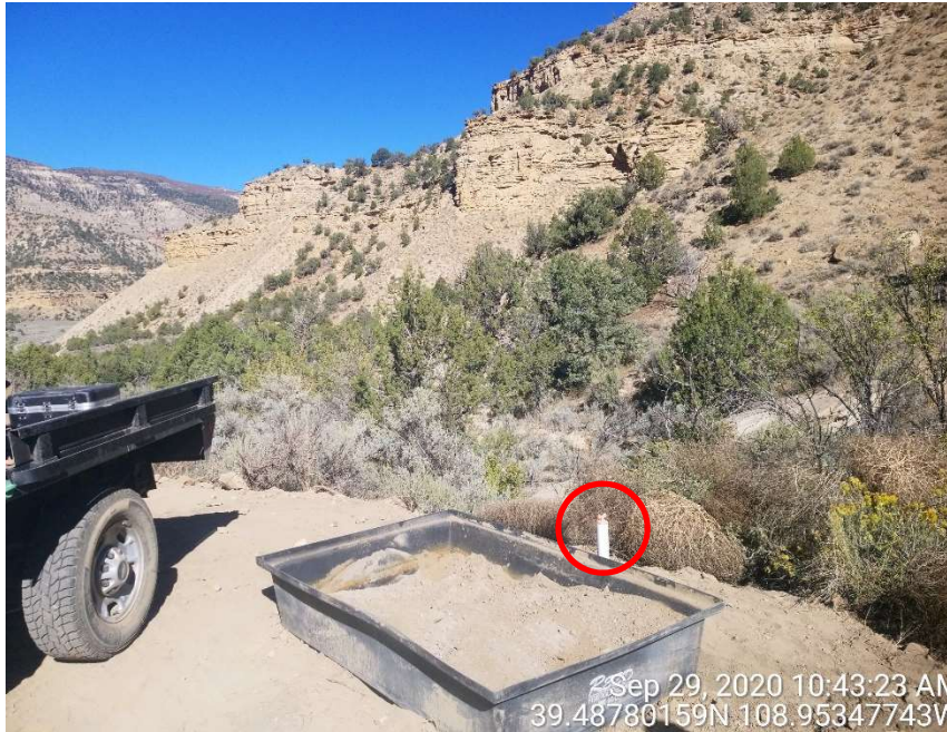
Newly installed monitoring well (red circle) and the arroyo located north of the location.
