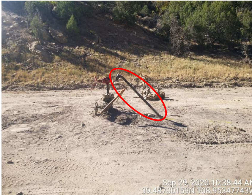
Wellhead, note the unmarked riser (red area).
