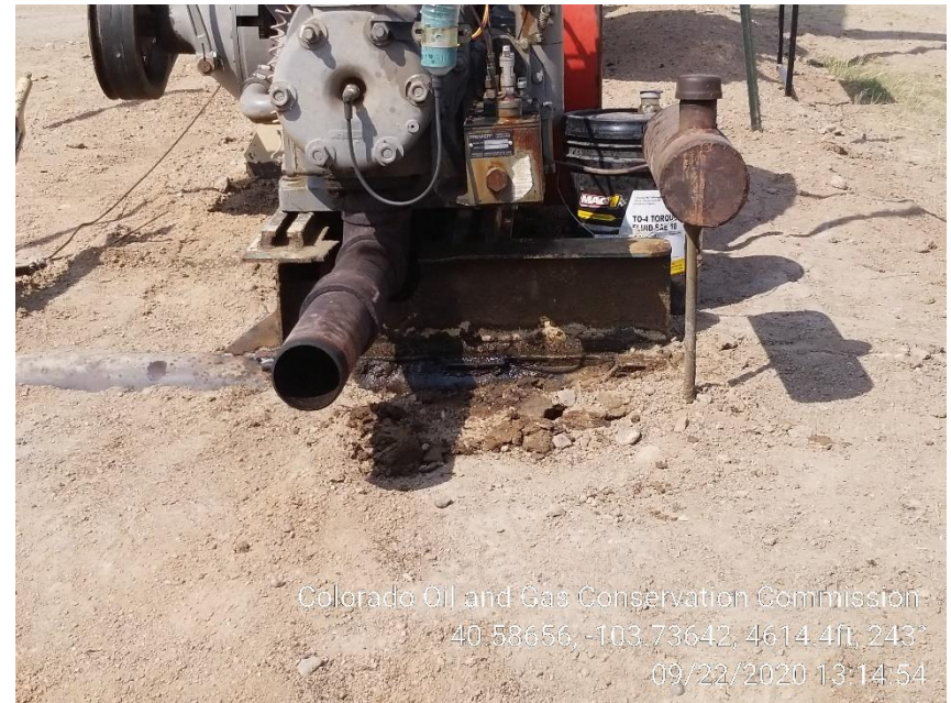
Photo 2 – Stained Soil at Gas Engine
