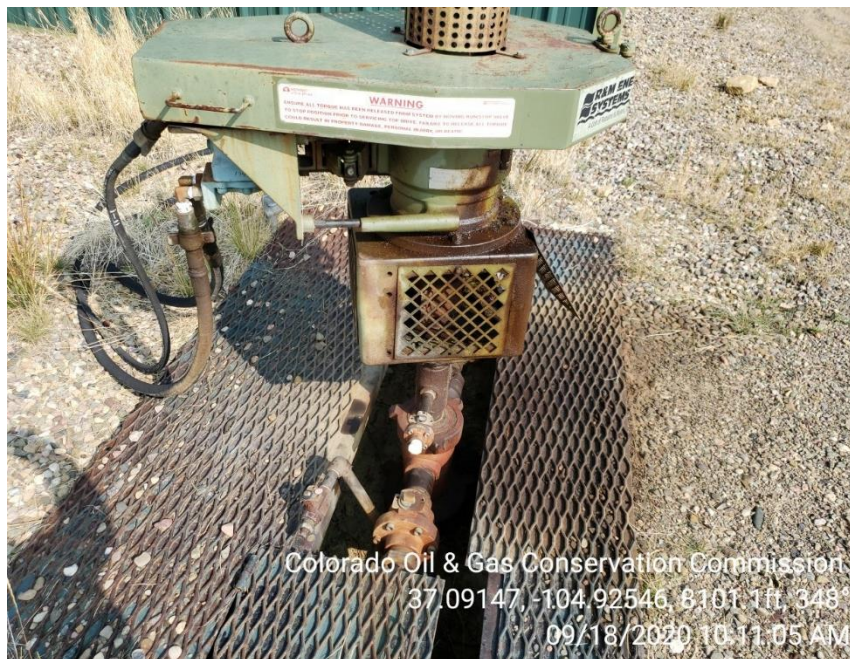
Photo 7 Wellhead with signs of oil leak
