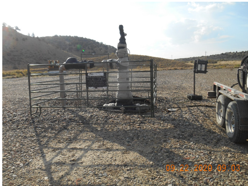
Injection wellhead
