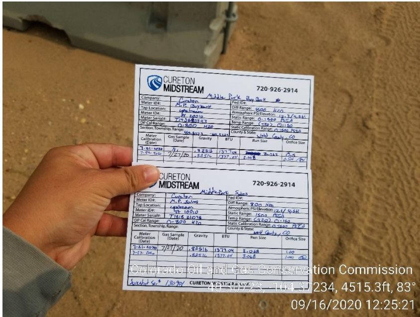
Photo 27 – Gas Meter Calibration Cards
