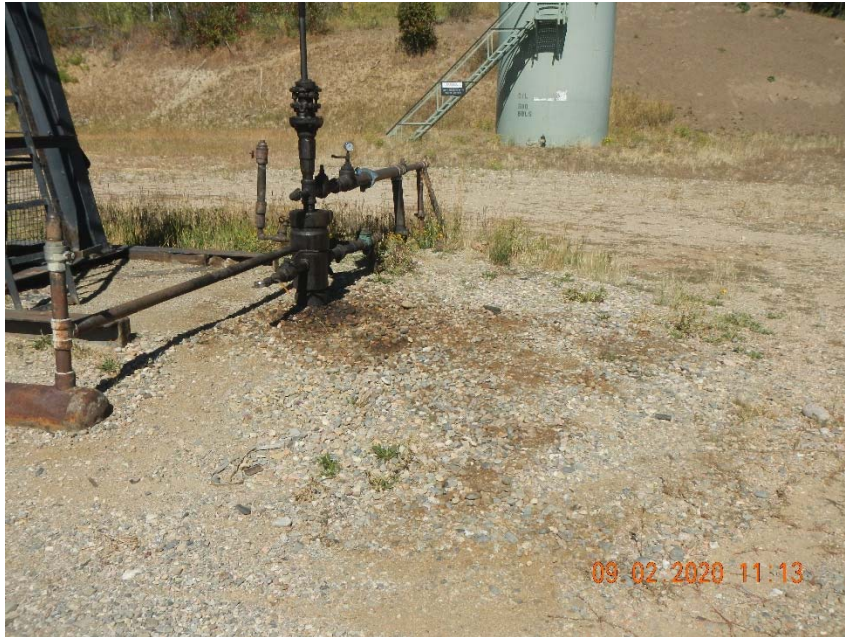
Photo 2. Stained soil at wellhead.
