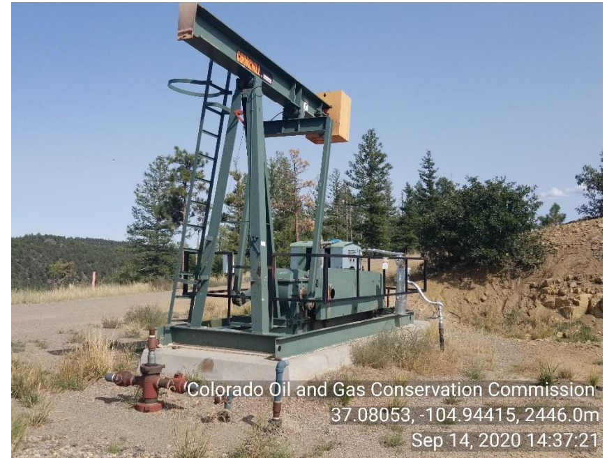
Photo 2 Unused equipment PU and risers not LOTO
