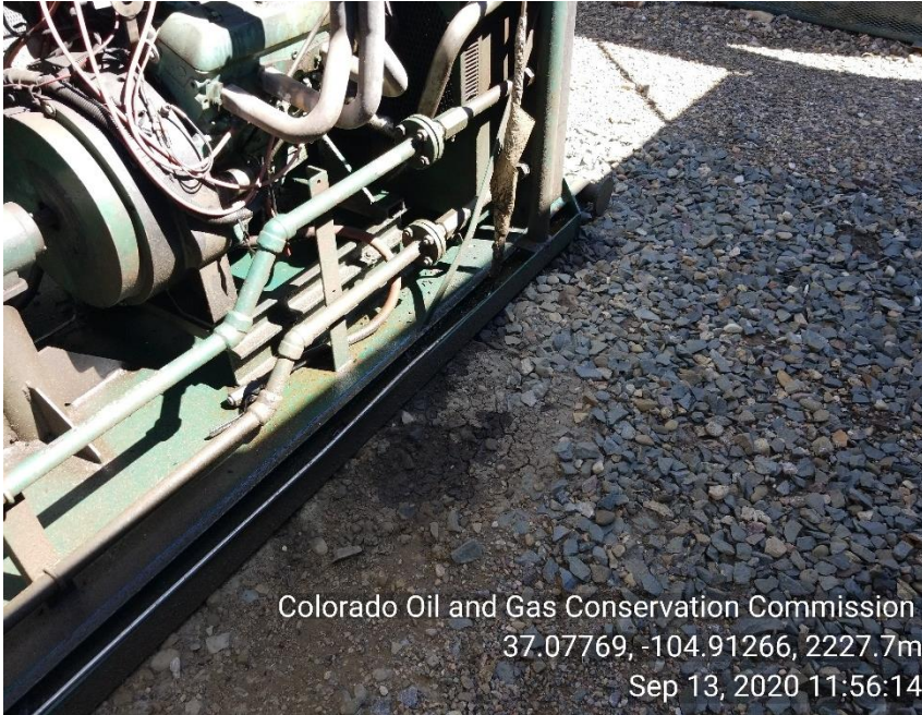
Photo 11 Stained soil around liquid ring.
