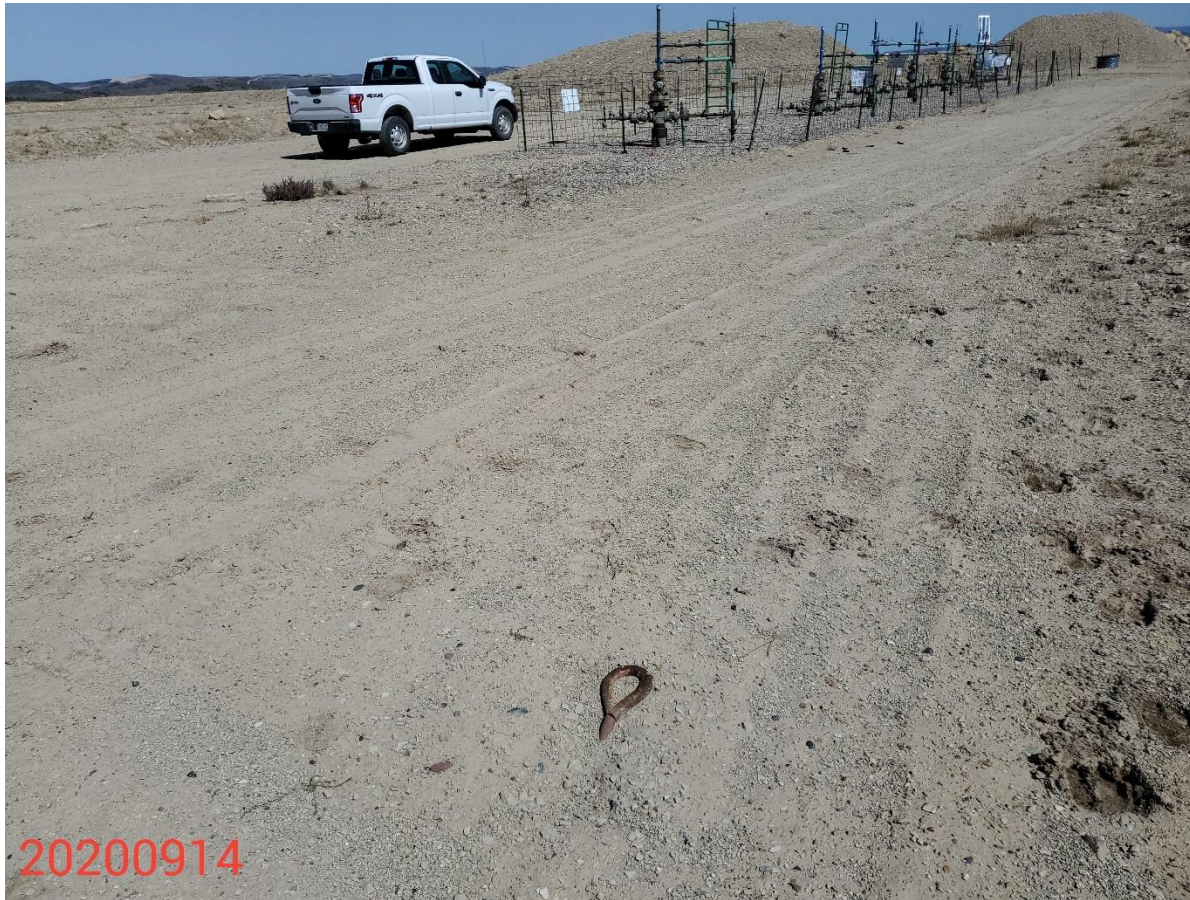
Photo 4: Photo shows example of guy line anchors observed on the Location without proper markers pursuant to Rule 1003.a
