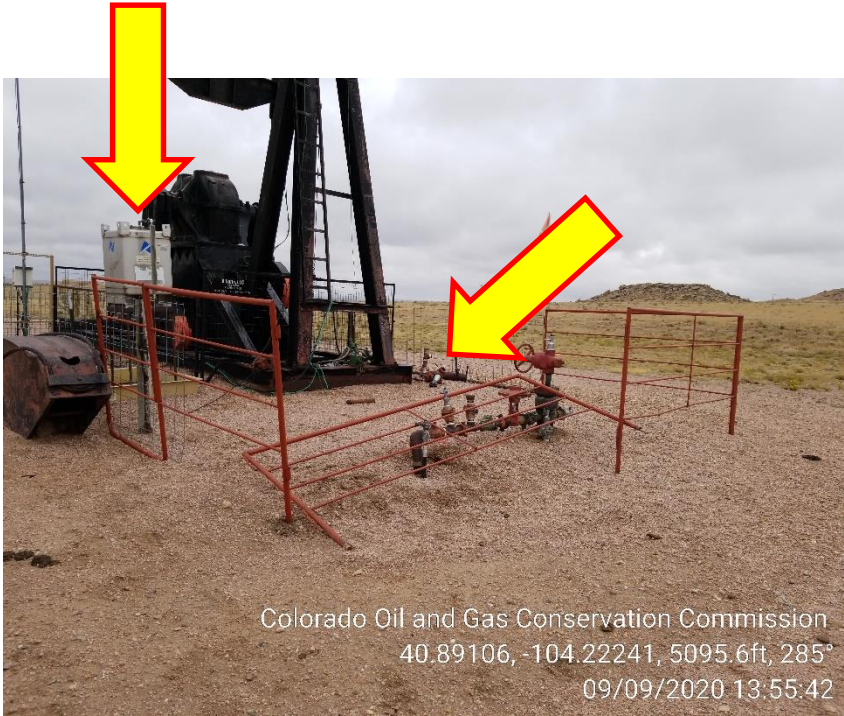
Photo 1 – Pumping Unit, Wellhead. Unused Chemical Tank, Pump, Stand and Containment. Unused Wellhead Parts
