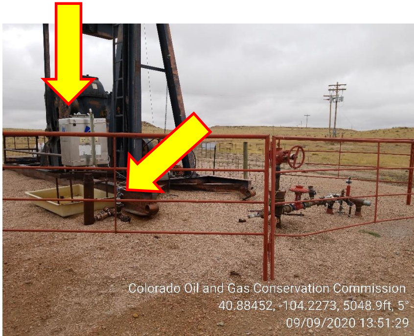
Photo 1 – Pumping Unit, Wellhead. Unused Chemical Tank, Pump, Stand and Containment. Unused Wellhead Parts
