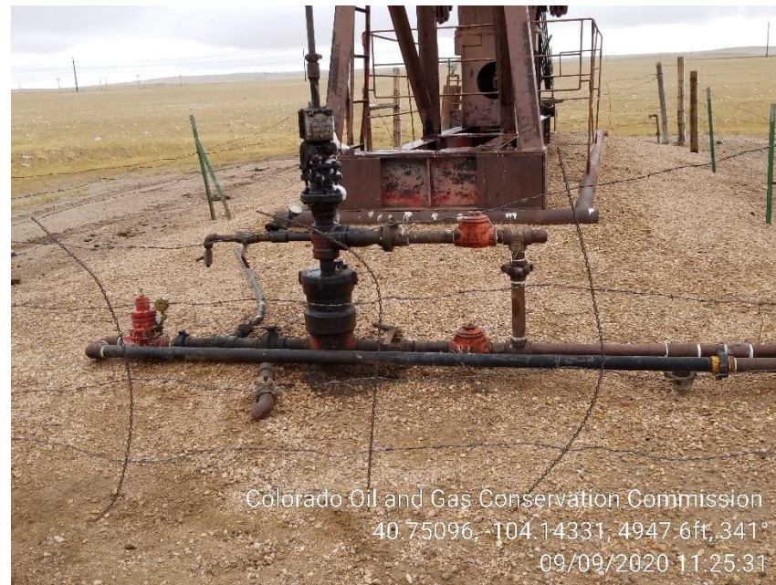
Photo 4 – Stained Soil at Wellhead
