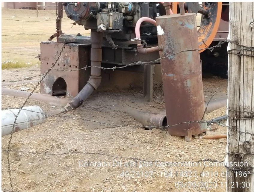
Photo 3 – Stained Soil at Gas Engine
