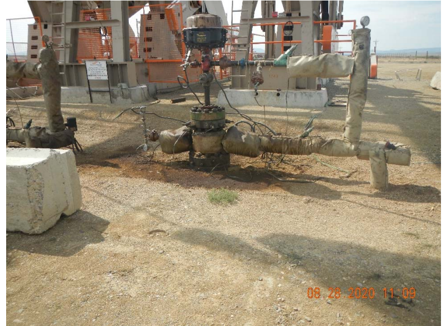
Photo 4. Stained soil at wellhead.
