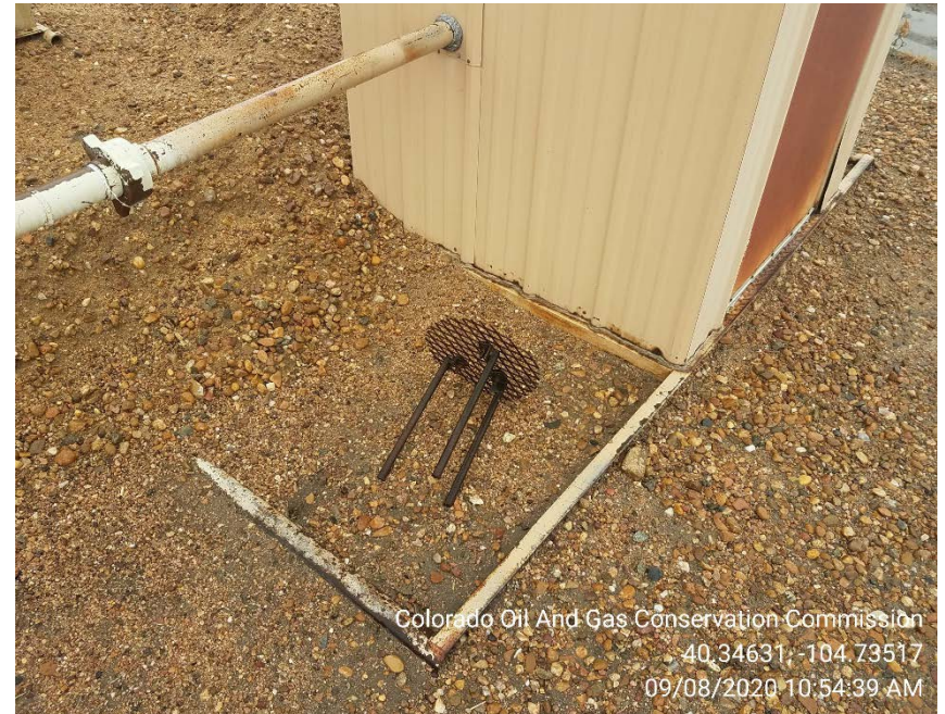
Separator burner stack wildlife screen
