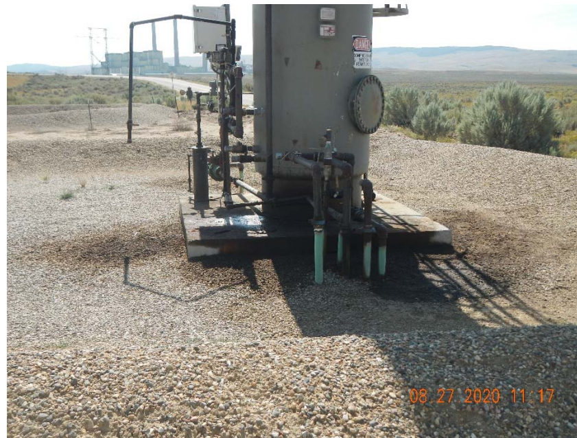
Photo 3. Stained soil at separator.
