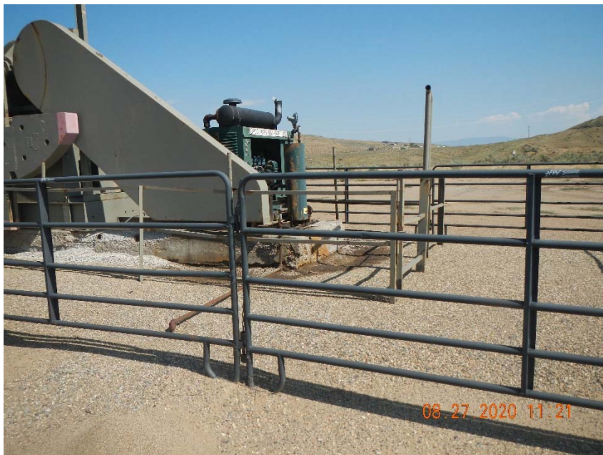
Photo 4. Stained soil at pump jack motor.
