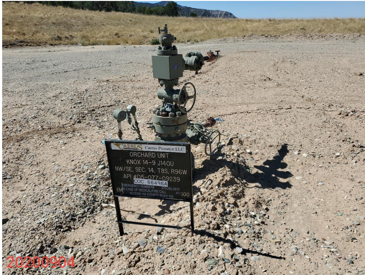
Photo 4: Photo shows only well remaining on the Location. Well status TA. All other production equipment has been remove from the Location.
