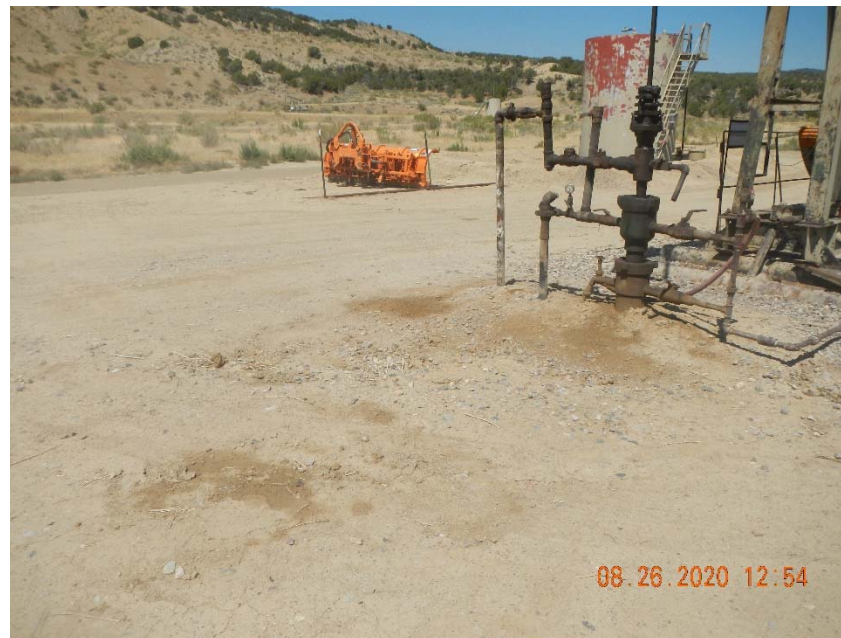
Photo 2. Stained soil at wellhead.
