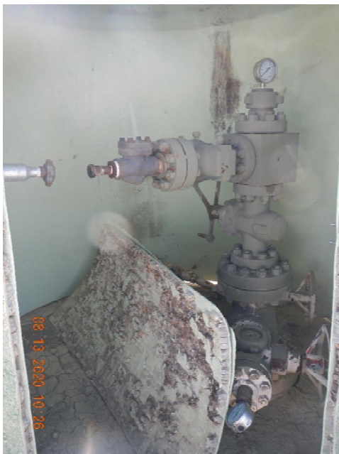
Photo 4. Photo of wellhead inside housing.
