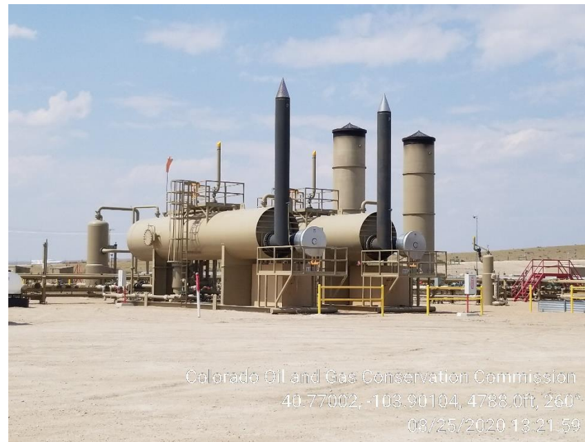
Photo 4 – Bulk Separators, ECDs
