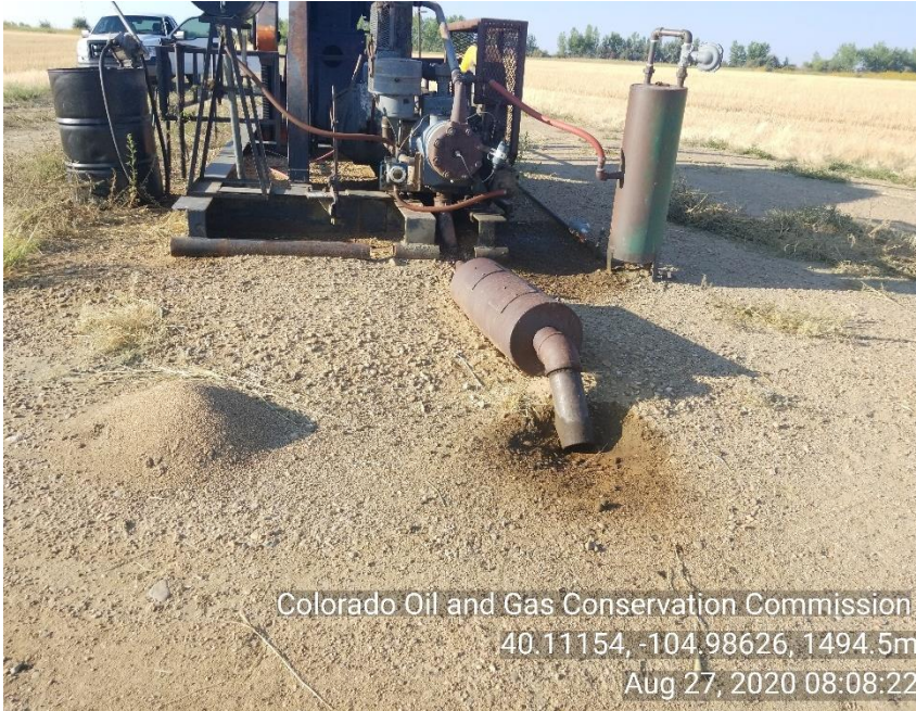
Photo 3 Stained soil around PU motor and exhaust pipe
