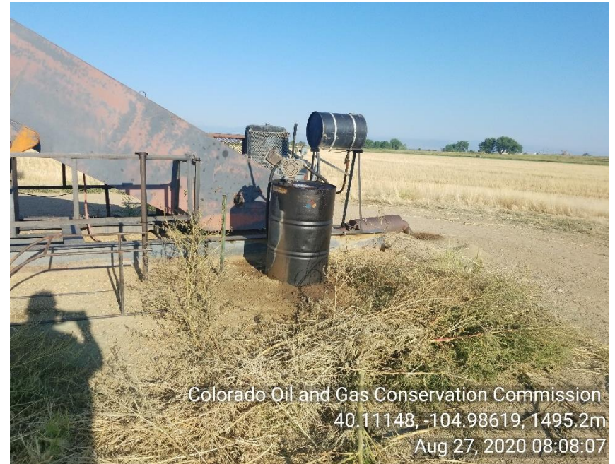
Photo 2 Improper fluid storage 55gal drum. Stained soil around 55gal drum.
