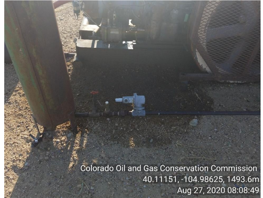
Photo 4 Stained soil around PU motor. Mechanical issue: stained soil appears to be coming from leaking PU motor.
