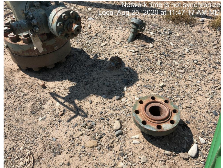
Photo #1781 Flow line riser not LO/TO.
