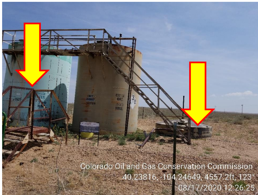
Photo 1 – Tank Battery. Produced Water Tanks missing NFPA Labels
