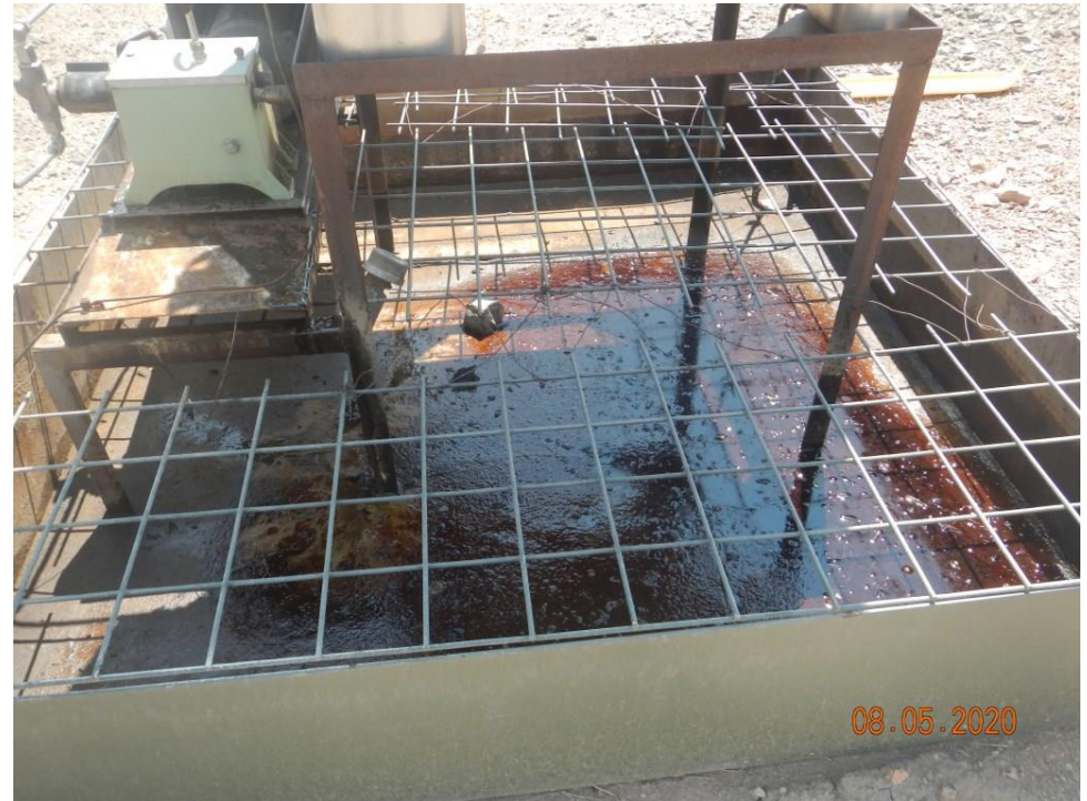
Photo#3: There is evidence of leaked fluids in containment.
