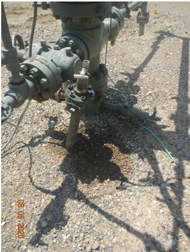
Photo#6: Staining at Well head.
