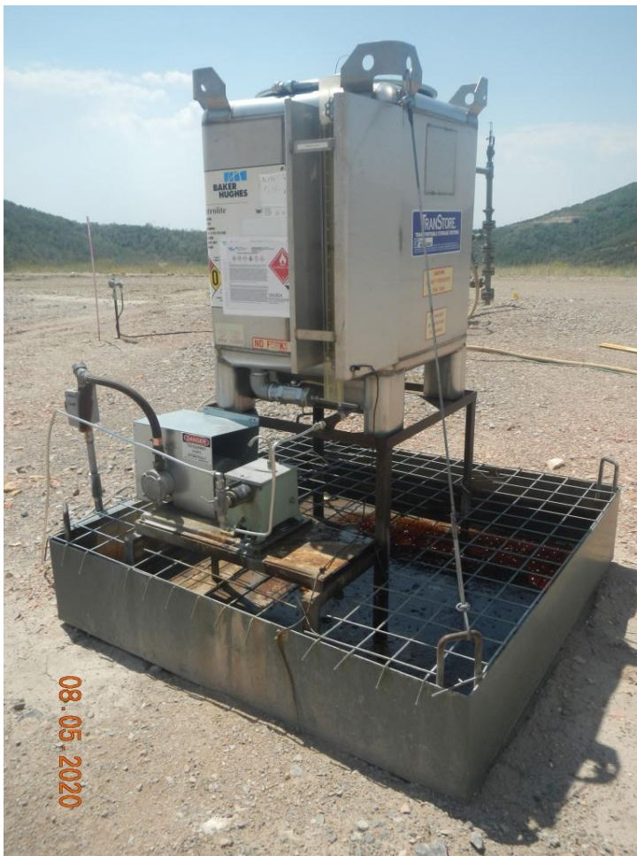
Photo#2: Secondary containment on equipment has hog panel as cover;
